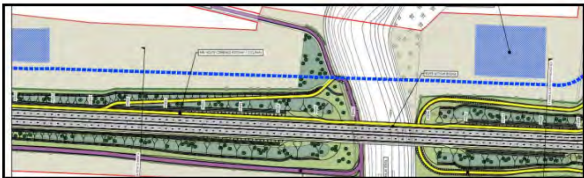
Figure 10: Example Construction Road Storage of Fladbury Soils
