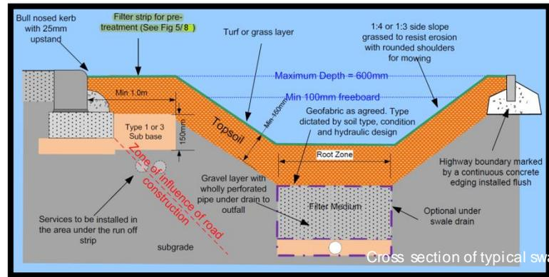
Suitable for all road types. Swales with infiltration must generally be a minimum of 5m from buildings (except for a permeable pavement that does not take any extra impermeable catchment such as a roof). Where they are less than 5m, the assessment should be approved by a suitably qualified professional such as a registered ground engineering advisor (See updated [\\*SuDS Manual \(C753\): Chapter 25 Infiltration](#) and [Susdrain Fact Sheet: Using SuDS close to buildings](#)).
