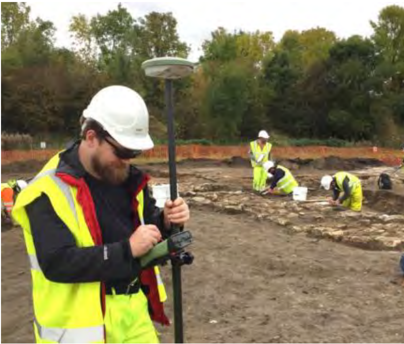
Plate 32: Investigation of tower, including DGPS survey; disused railway with trees in background
